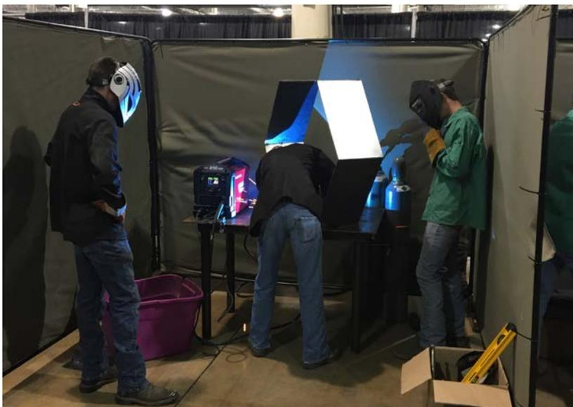
*Each team was required to incorporate 5 SMAW welds, 5 GMAW welds and 5 oxyfuel cuts in the design of their project. Welds were performed with a Lincoln Electric POWER MIG® 210 MP welder.*
