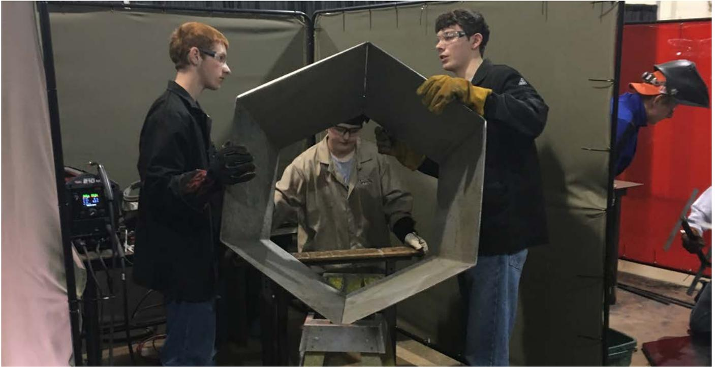
*Teams of three students had three hours to fabricate, weld and finish their fire pit from pre-cut parts during the Ohio FFA welding competition.*
